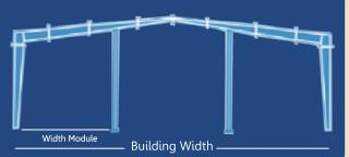
Section design of frame is optimized, flexibility in section member fabricated from standard section / built up sections. Frame can be designed for future expansion.
